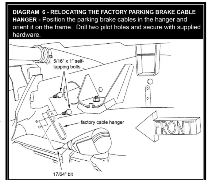
driver side parking brake cable in the lower hole in the "03" bracket. Be sure the prongs of the factory cable retaining clips are spread enough to secure each cable.
