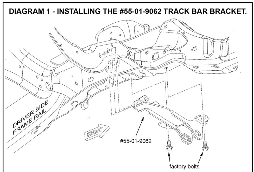
Often there is an excessive amount of undercoating build-up on the crossmember, especially on the back (rearward facing) portion of the crossmember where the undercoating has pooled up. Scrape off any excessive undercoating to prevent the track bar bracket from loosening over time.
