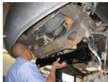
Two full-width crossmembers stoutly mount the lower A-arms
